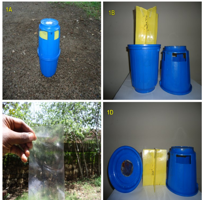
A: sticky trap assembled as operative; B: top part of trap with removable quadrants/panels where adhesive plastic sheet attached; C: adhesive plastic sheet with trapped mosquito; D: disassembled trap
