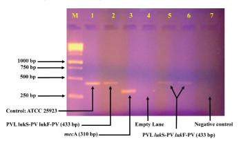
Lane M shows molecular marker; Lane 1: positive control ATCC (25923); Lane 2,5,6 shows *lukS*/F-PV (433bp) and lane 3 shows *mec*A (310bp); Lane 7: negative control DNA free water.
