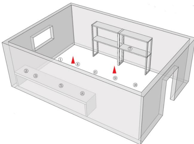
Locations ①, ④, ⑥, ⑨, and ⑩ were on the floor, while locations ②, ③, ⑤, and ⑧ were on a table, ⑦ was on a shelf. All the locations were approximately 0.7 m above the floor. ▲ represents the locations of the UV-C disinfection device.
